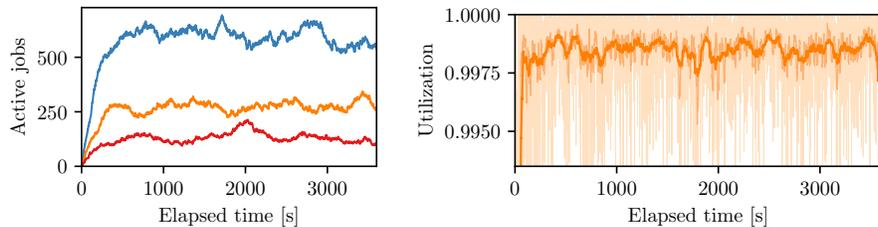
**Fig. 5.** Left: Number of active jobs for interarrival times  $1/\lambda$  of 2.5 s (top), 5 s (middle), and 10 s (bottom). Right: System utilization (i.e., ratio of busy PEs) for  $1/\lambda = 5\text{ s}$  at a sliding average of window size 1 s, 15 s, and 60 s respectively.
