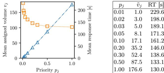
**Fig. 4.** Impact of job priority on mean assigned volume (left axis, blue triangles) and response time (right axis, orange squares). The table shows the used priorities  $p_j$  with the corresponding mean assigned volume  $\tilde{v}_j$  and mean response times in seconds.
